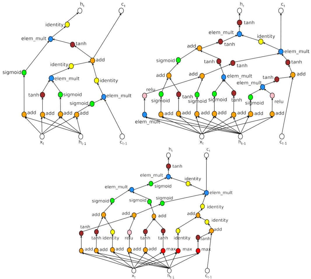
Figure 8: A comparison of the original LSTM cell vs. two good cells our model found. Top left: LSTM cell. Top right: Cell found by our model when the search space does not include *max* and *sin*. Bottom: Cell found by our model when the search space includes *max* and *sin* (the controller did not choose to use the *sin* function).
