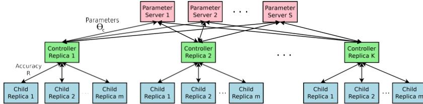
Figure 3: Distributed training for Neural Architecture Search. We use a set of 5 parameter servers to store and send parameters to  $K$  controller replicas. Each controller replica then samples  $m$  architectures and run the multiple child models in parallel. The accuracy of each child model is recorded to compute the gradients with respect to  $\vartheta_c$ , which are then sent back to the parameter servers.
